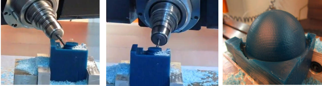
Figure 4.2 Using NX Post processor to drive Fryer 5X machining center to make a wax part
